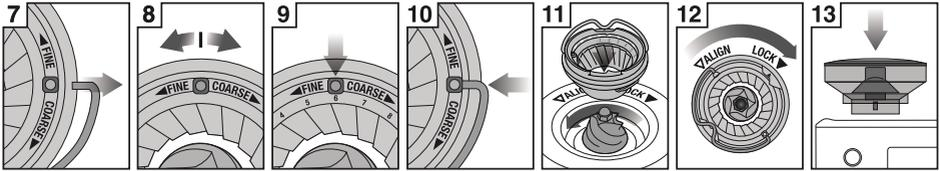
7 Remove wire handle from both sides of the burr      8 Move adjustable top burr, 1 number, coarser or finer      9 Align the number with the handle opening      10 Insert wire handle from both sides of the burr      11 Push upper burr firmly into position      12 Lock upper burr      13 Align hopper into position
