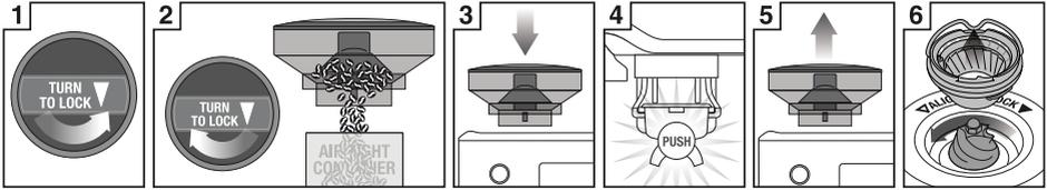
1 Unlock hopper      2 Hold hopper over container & turn dial to release beans into container      3 Align hopper into position      4 Run grinder until empty      5 Remove hopper      6 Remove upper burr
