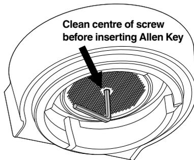
5. Once loosened, carefully remove and retain the screw, stainless steel shower screen. Make note of the side of the shower screen and dispersion plate that are facing downwards. This will make re-assembly easier. Wash the shower screen in warm soapy water, then dry thoroughly.
