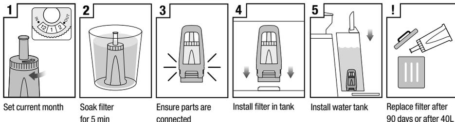
The provided water filter helps reduce the risk of scale build-up in and on many of the inner functioning components. Replacing the water filter every three months or 40L will reduce the need to descale the machine.
